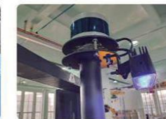
视觉系统 | Visual system 基于雷达的二次定位,整体定位精度可达10mm。 Based on radar secondary positioning, the overall positioning accuracy can reach 10mm.
