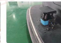
雷达系统 | Radar system 全向雷达,采用自然导航,无需调整基础设施,具备超高环境适应能力。 Omnidirectional radar, using natural navigation, no need to adjust infrastructure, with high environmental adaptability.
